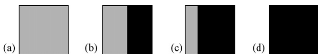
Fig. 10. Variation of the backings for the four different MEAs, which results are shown in Figs. 9 and 10. The gray areas are marked the GDL with a low hydrophobicity, the black area the GDL with the strong hydrophobicity. The cathodic gas inlet is on top left, the used flow field in a serpentine flow field where the channel go up and down from left to right. The gas outlet is on bottom on the right side.
